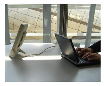
The Altai C1an employs patented smart signal processing algorithms and antenna design to increase Wi-Fi signal strength (transmit and receive) by as much as 18 dB in areas covered by an A8n Super WiFi Base Station or A2 WiFi Access Point. It can be installed exactly where the throughput is required to boost up, and it allows the service operator to increase the coverage range of an A8n base station substantially and provides greater flexibility and cost savings to Wi-Fi deployments.
