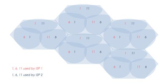
The above illustration can also be looked as a mixed type of sector and omni coverage AP. For example, each hexagon is a large cell site covered by three sector APs by ISP 1. Each hexagon also represents three small cell sites each covered by one omni AP by ISP 2.
