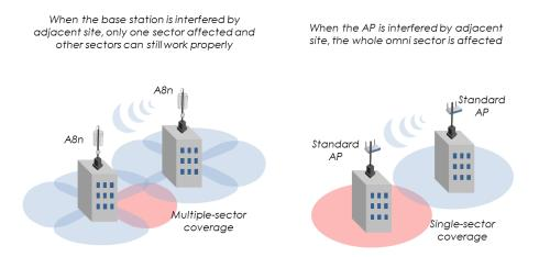
If the omni coverage design of the multiple radios AP is changed to sector coverage design, the interfering direction can be narrowed down more precisely and the affected area can be reduced. This can be illustrated in below by using the Altai A8-Ein Super WiFi base station as an example.
