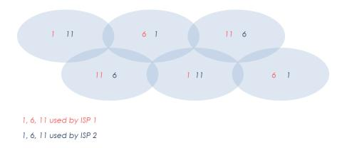
For sector coverage type of AP or base station, the frequency planning for two networks with minimum interference can be shown below:
