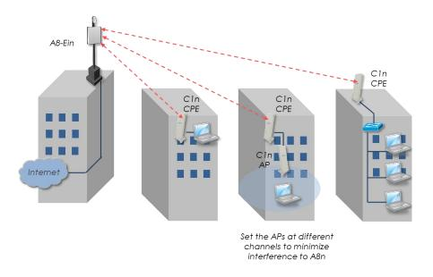
The A8n – C1n combination can be fully utilized in different rural wireless broadband scenarios to provide indoor or extended outdoor coverage.
